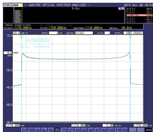
Swept laser spectrum at 1310nm.
