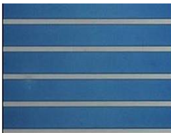
Optical microscope image of 20 μm lines imprinted on InP. Protrusion coverage is 20%
