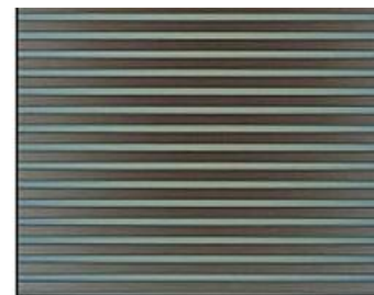
Optical microscope image of 20 μm lines imprinted on InP. Protrusion coverage is 40%
