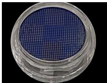
Photograph of imprinted Ø50mm Indium Phosphide (InP) wafer. All imprinted structures are 20 μm lines. The protrusion coverage varies from 20% to 60%
