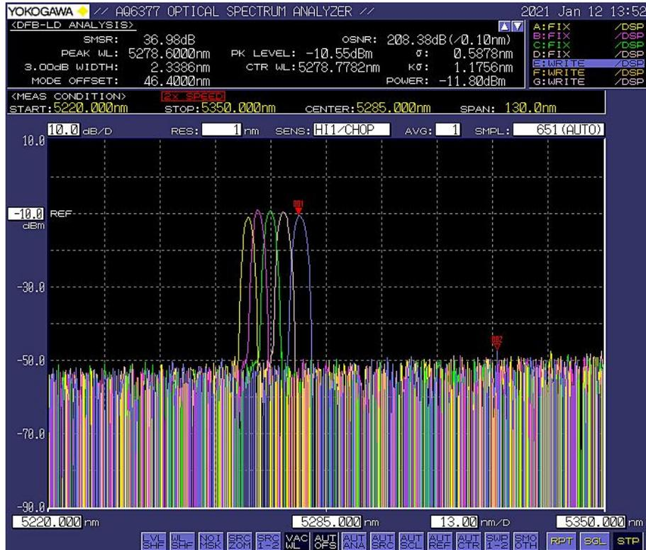
黄线: 150mA,5267.08nm; 红线: 165mA,5269.48nm; 绿线: 180mA,5271.52nm;
